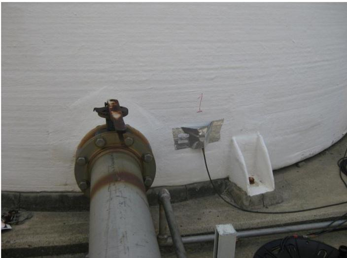
Figure 2 – An Installed Acoustic Emission Sensor
