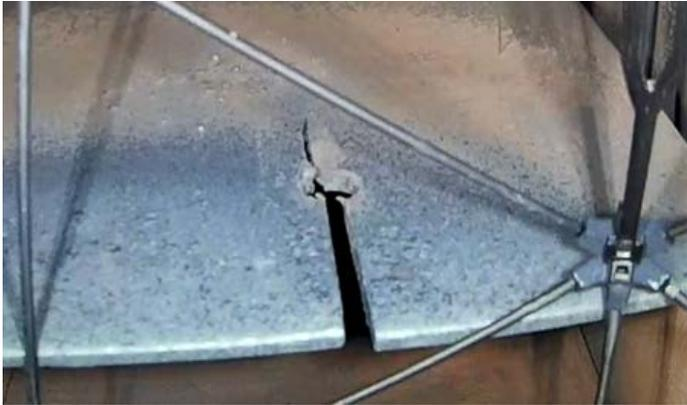
Figure 2: Visible Cracking detected from the RPA
