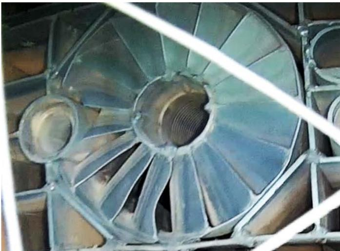
Figure 3: Distorted Burner Elements visible from the RPA
