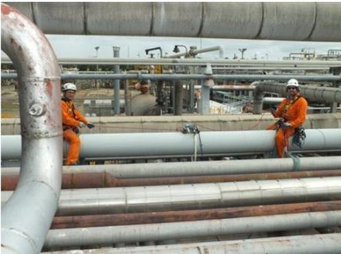
Rope Access Technicians pulling a SLOFEC scanner along a pipe
