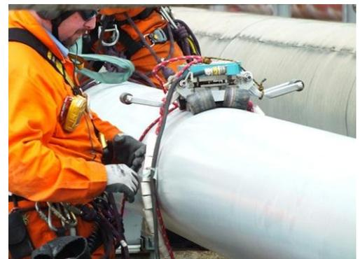
SLOFEC equipment secured with a safety lanyard
