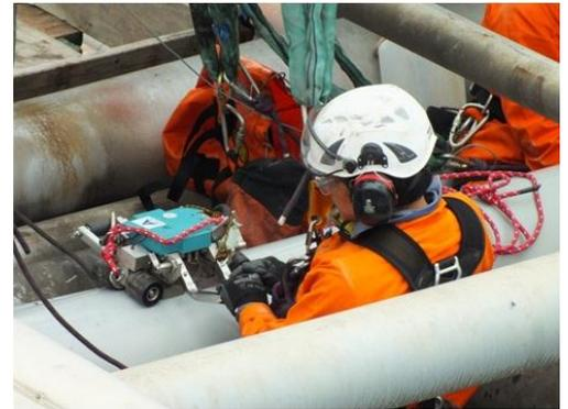
Rope Access Technician using a SLOFEC scanner
