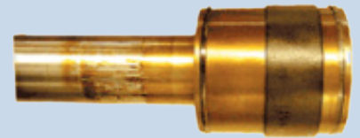
Figure 1: Varnish Formation on Valve
